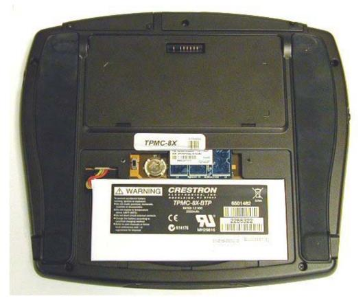
**TPMC-8X-BTP** in Battery Compartment of **TPMC-8X**
